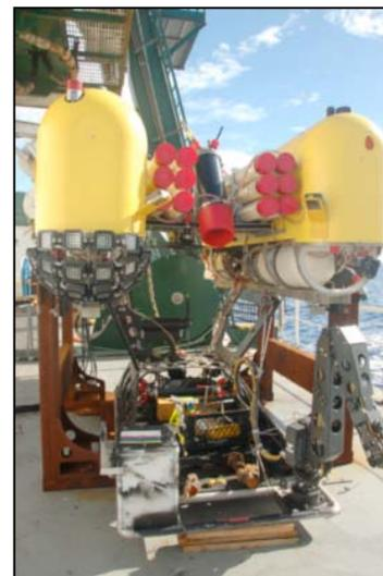
**Figure 1.** The newly-developed *Nereus* in ROV mode in May 2009 showing ceramic pressure housings, lateral and vertical thrusters, ROV-mode flotation spheres, robotic arm, digital imaging cameras, and LED lighting arrays.
